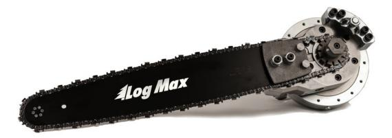
The key component of the True-Cut system is the intelligent saw motor with integrated valving solutions for saw motor speed and saw bar control. The True-Cut saw maintains an almost constant chain speed of 40 m/s throughout the cutting cycle.
